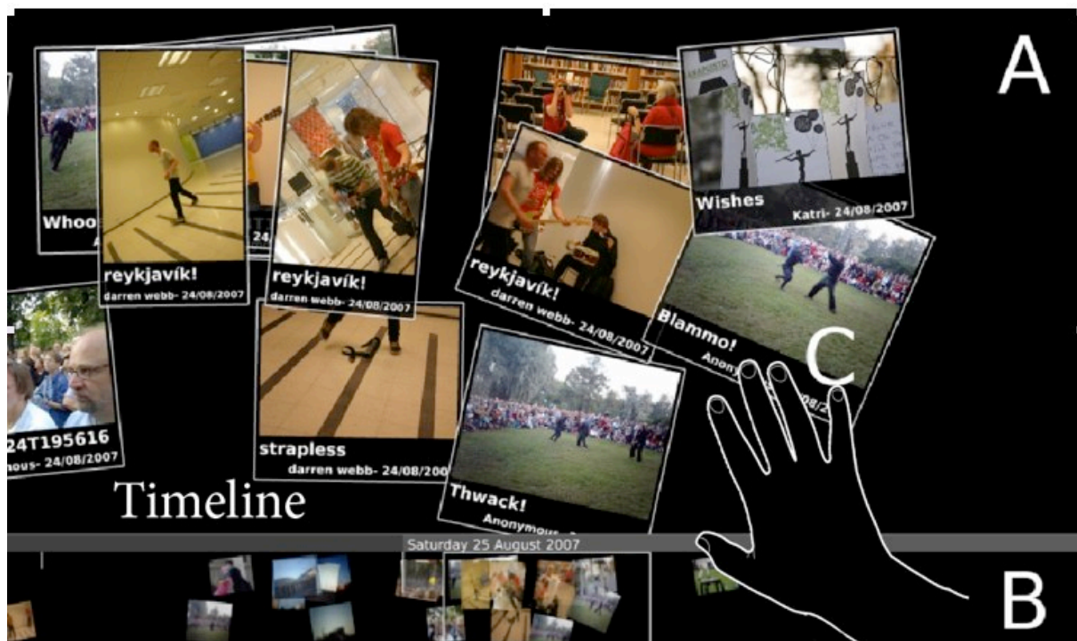
Figure 2: CityWall user interface: the content area (A), scrollable timeline (B) and picture content (C).
