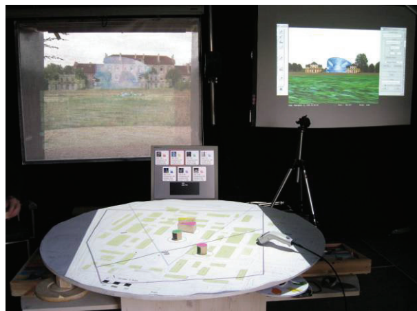
Figure 6: The technical setup inside the MR Tent is centered around the two projection walls and the projection table
