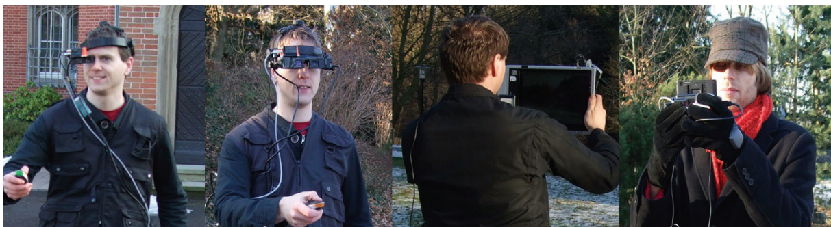
Figure 32: Compared devices: monocular and binocular see-through display (left) and Tablet PC and UMPC (right).
