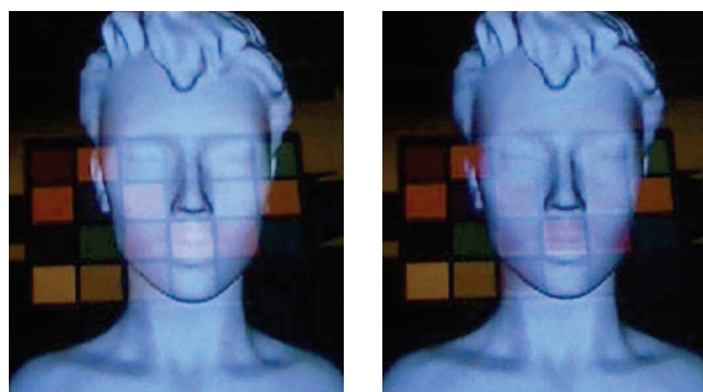
Figure 31: Images captured by a webcam through the see-through display. Left is the uncompensated image, the right one is compensated with Subtraction Compensation.
