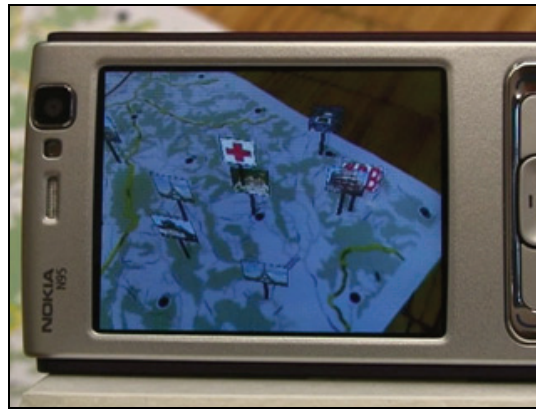
Figure 9: Map tracker running on a Symbian device (Nokia N95) displaying a simple augmentation registered in 3D onto a dotted map.
