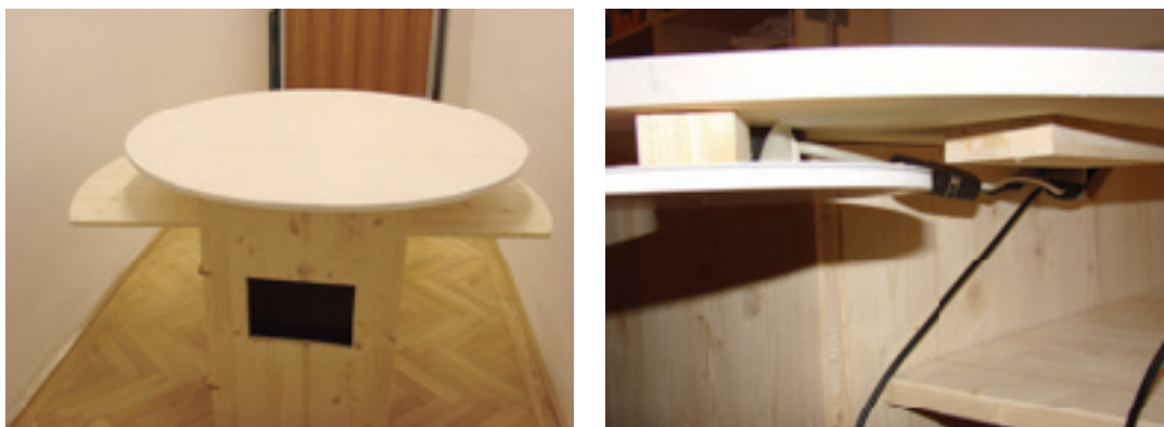
Figure 10 - Physical ColorTable; including rotating viewpoint, tangible selector and barcode reader
