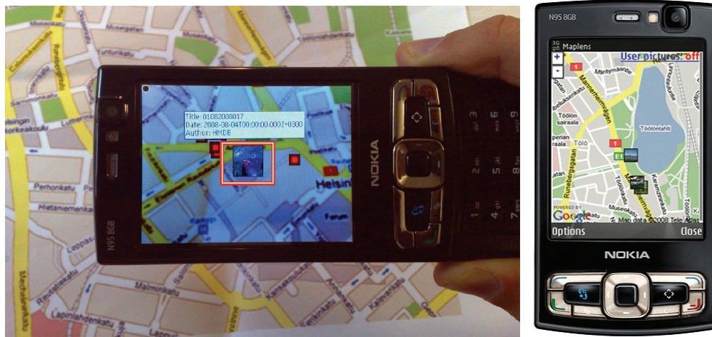
Figure 2 Left MapLens in use with a paper map, overlaying digital information on screen. With the red square (centre) user locates and selects markers—as one user states—“catches them”. Right DigiMap version, Google Map with markers
