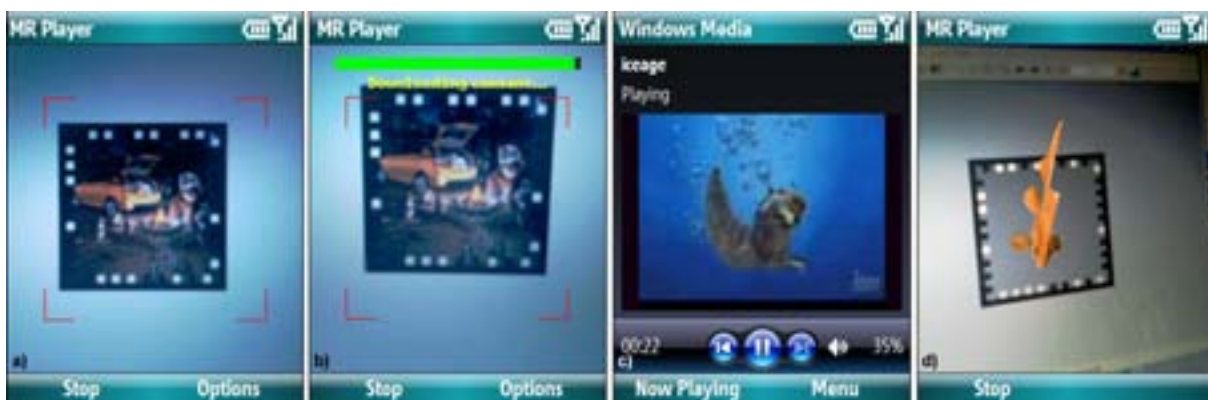
Figure 19: Screenshots of the MR-Player application in use: a) User points the camera at a visual marker. b) Content is downloaded from the server. c) Video playback. d) 3D geometry presented overlaid onto the marker.
